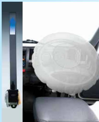
*SRS airbag system and seat belt with pretensioner are activated in the event of a frontal collision, mitigating impact to the head and chest.
