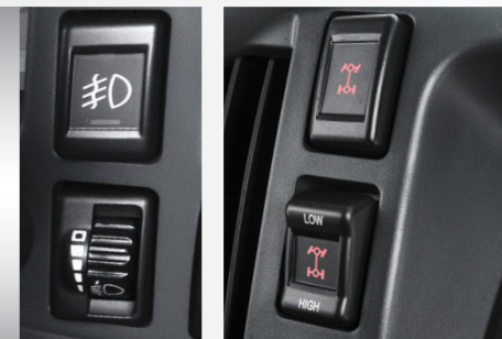
Headlight leveling. Preferred headlight beam position can be maintained when truck is loaded and when it has no load
