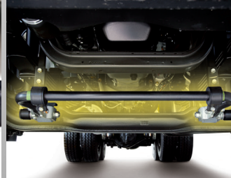
▲ Stabiliser Bar (Applicable to FXZ77UU-M).
