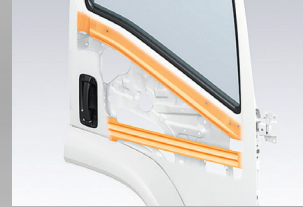
▲ Door impact beam with high tensile strength reinforcement frame.
