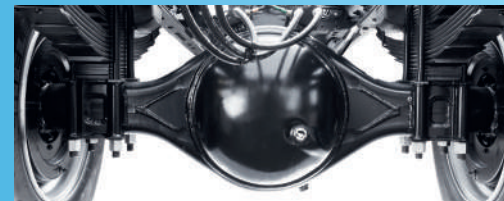
Bigger rear axle for higher load capacity (13 ton).
