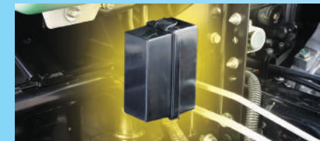
Electrical relay box positioned higher to avoid damages from flood.
